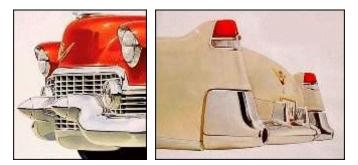
The bumper impact guards and the jet-like exhaust outlets
